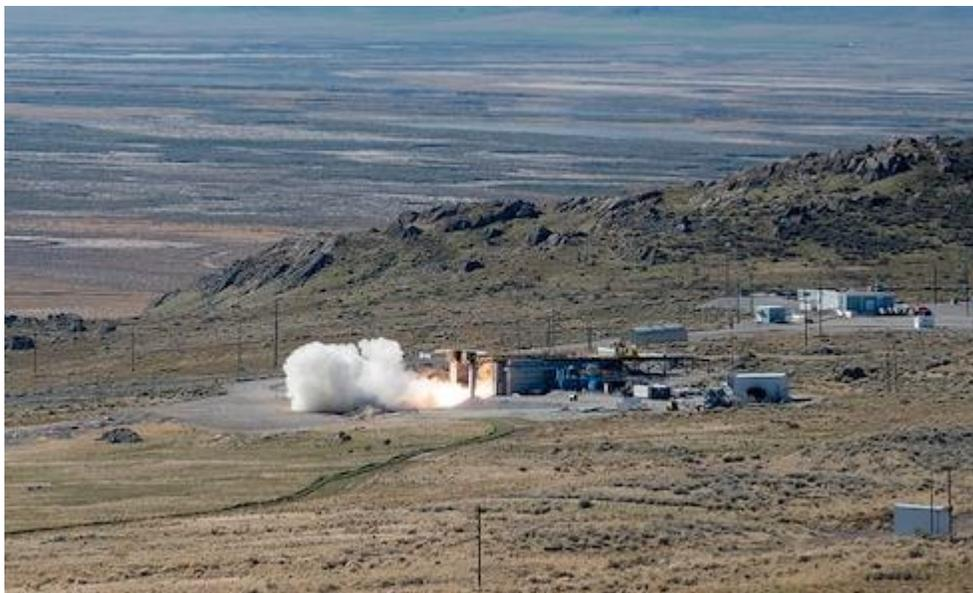
PROMONTORY, Utah (Oct. 29, 2021) The U.S. Navy, in collaboration with the U.S. Army, conducts a static fire test of the first stage of the newly developed 34.5" common hypersonic missile that will be fielded by both services. (U.S. Navy photo courtesy of Northrup Grumman)
