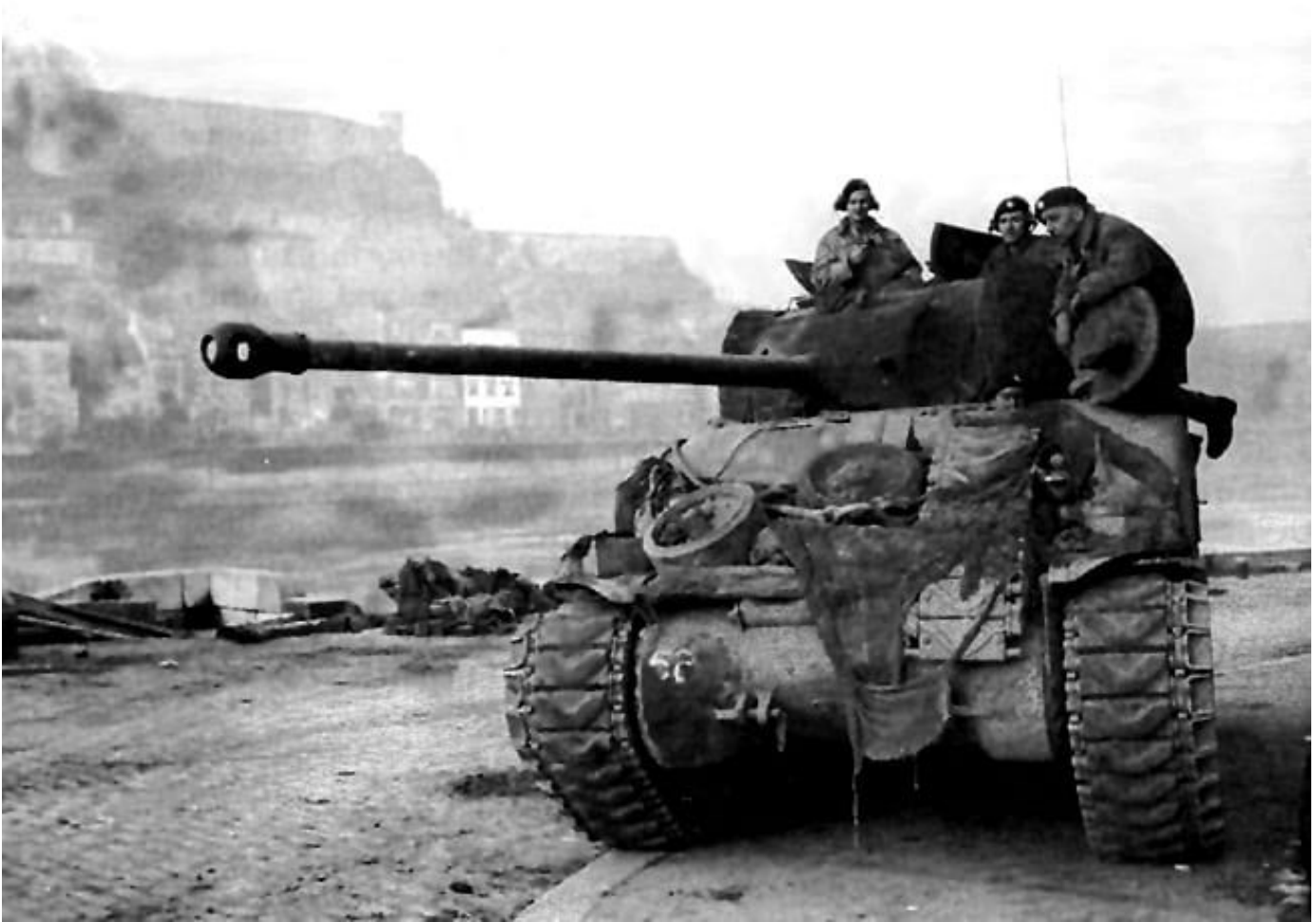
A British Sherman Firefly patrolling the Meuse at Namur in 1944. The Firefly was a British attempt to give the Sherman a better chance against German Panthers and Tigers by upgunning it with a 17-pounder instead of the typical 75 mm low velocity gun. The assortment of road wheels, lengths of track, sandbags and wooden planks often piled on the exteriors of M4s reflects the degree of the crews' confidence in their armor protection. Photo courtesy of the U.S. Army Center of Military History
