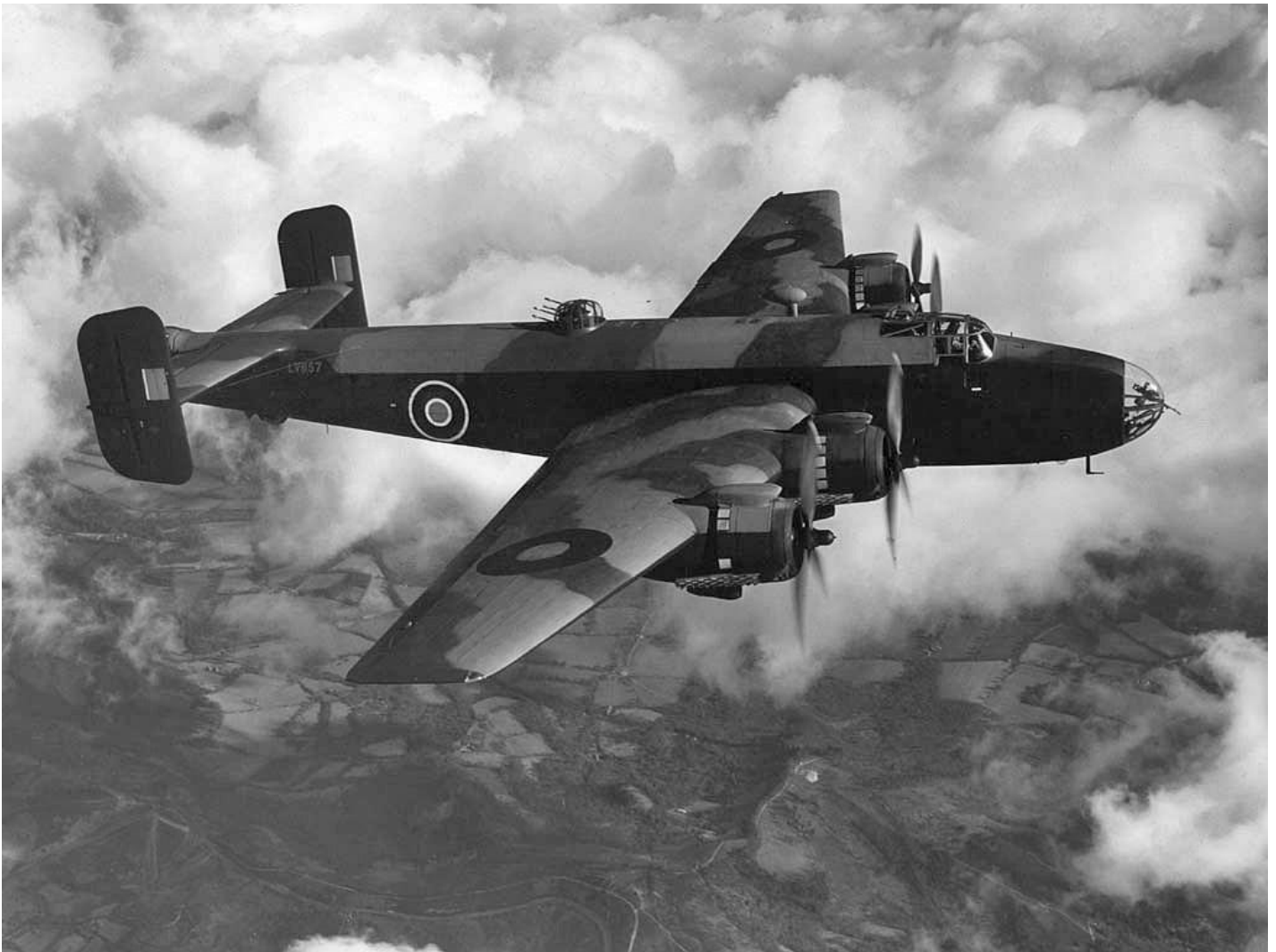
A Halifax B Mk. III, with its distinctive square tailfins and Bristol Hercules radial engines. The Halifax was the second major heavy bomber in the Berlin raids, and, with the Stirling, was gradually pulled from front-line operations. Royal Air Force photo
