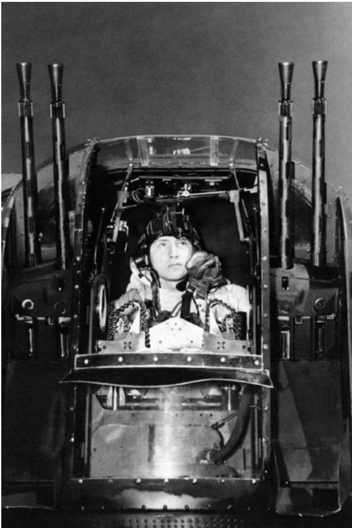
A Lancaster tail gunner in his Frazer Nash turret with four .303 machine guns. He is behind a “clear vision canopy” which is semantics for having nothing between him and lurking night fighters but the below freezing blackness of the night sky. IWM photo
