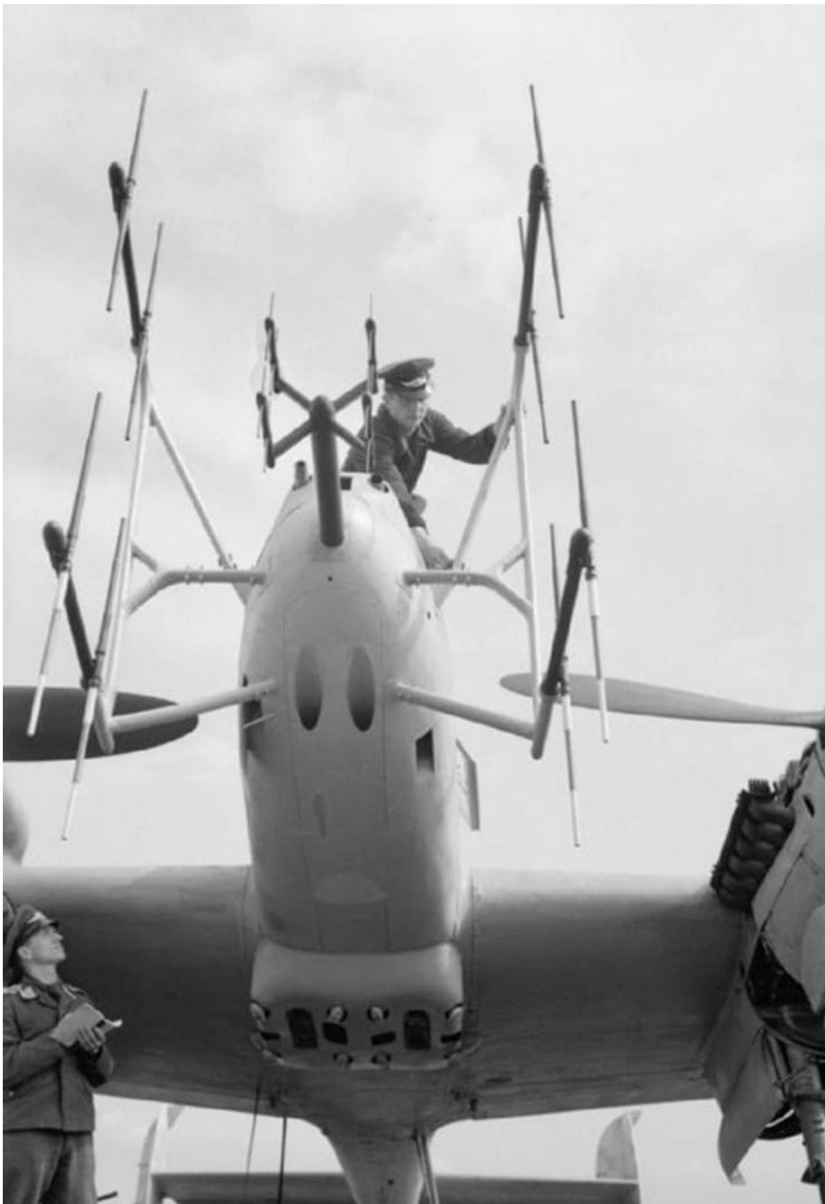
FuG 220 SN-2 and FuG 202 B/C (center) "Lichtenstein" night fighter radar equipment on the nose of a Messerschmitt Bf 110G-4. The older B/C radar was retained for short-range acquisition of targets until the SN-2's minimum range performance was improved. IWM photo
