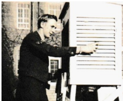
At the Selfridge Field instrument shelter, Sgt. George Popadines turns a crank hidden by his hand. It will twirl a thermometer mounted inside. To promote evaporation, a water-soaked gauze covers the thermometer's end. After twirling, the thermometer will show a "wet bulb temperature" reading, 1949.
